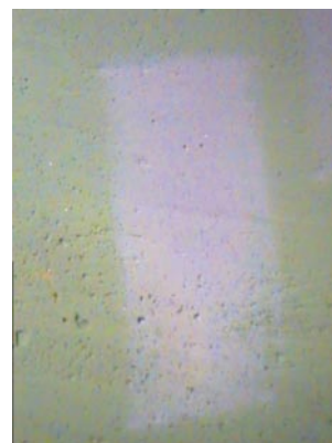
Fig. 3 Optical micrograph of irradiated \text{Cr}_2\text{O}_3 powder, fluence 0.5\text{ J cm}^{-2} , showing a silver-metallic rectangular mark. The mark is approximately 3 mm wide and 7.5 mm high.
